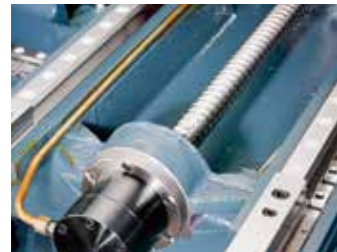
/ BALLSCREW COOLANT SYSTEM
