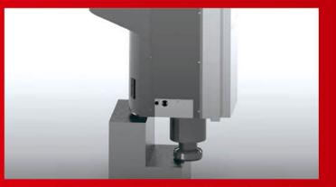
KAFO adopting long nose spindle, suitable for die & mold and specific parts cavities avoids interference during processing. it is able to mount all kind of angular milling head (option)
