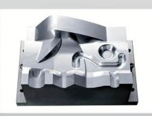
**TESTING WORKPIECE** Benz Mold sample
