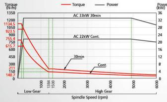
**/ BT50** GEAR HEAD 6000 RPM (HEIDENHAIN OAN260L) - Torque - Powe
